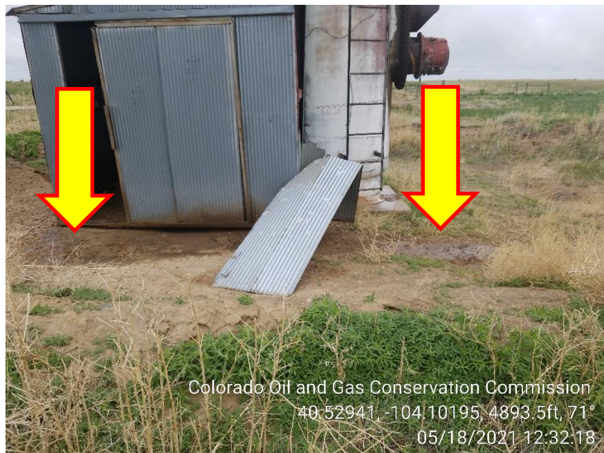
Photo 7 – Stained Soil at Heater Treater
