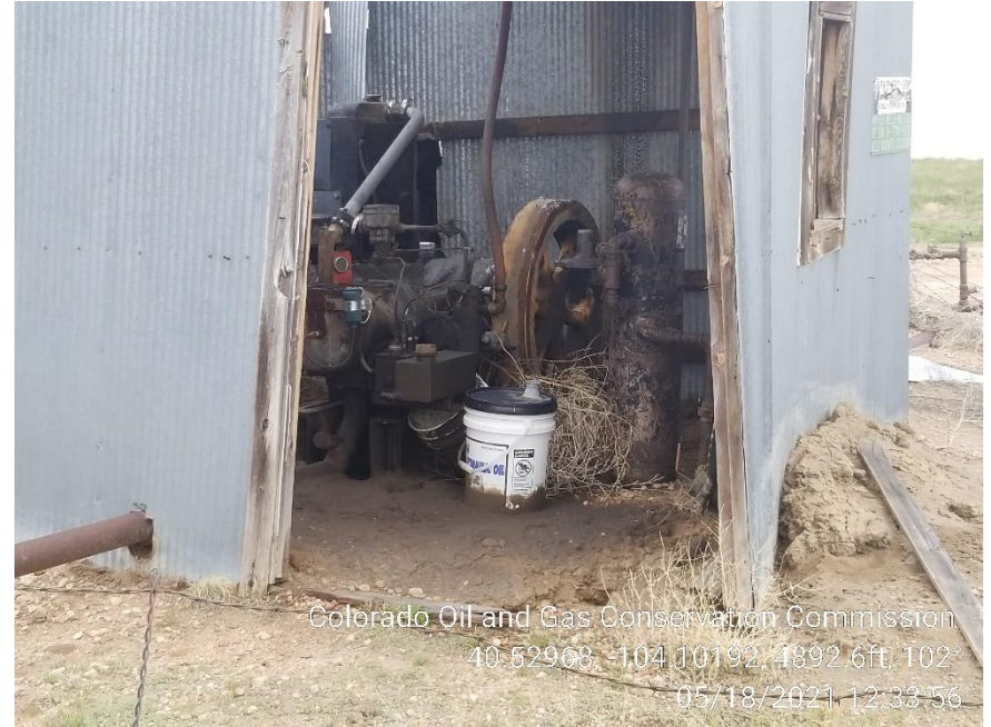
Photo 14 – Stained Soil at Gas Engine
