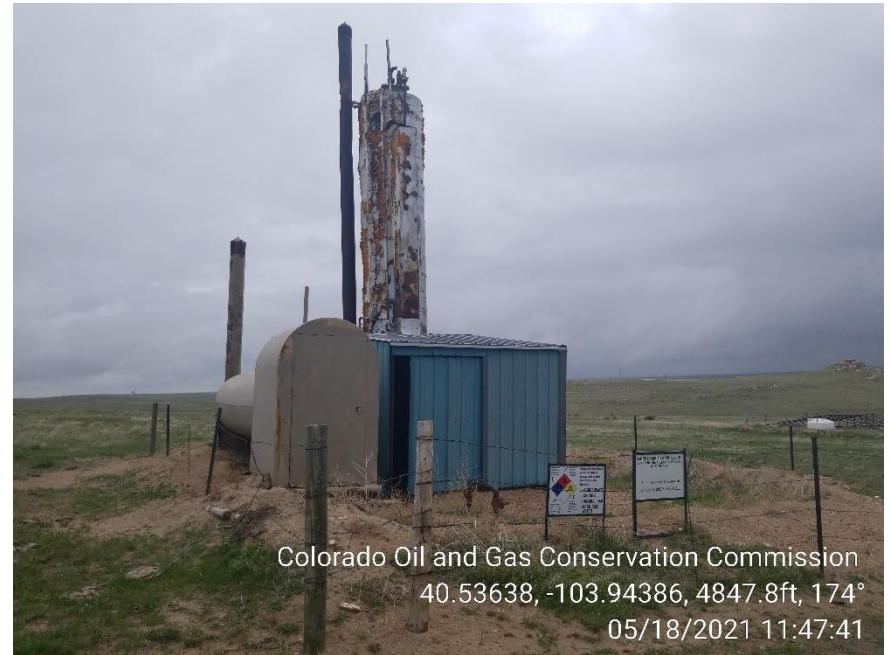
Photo 4 – Heater Treater and Separator
