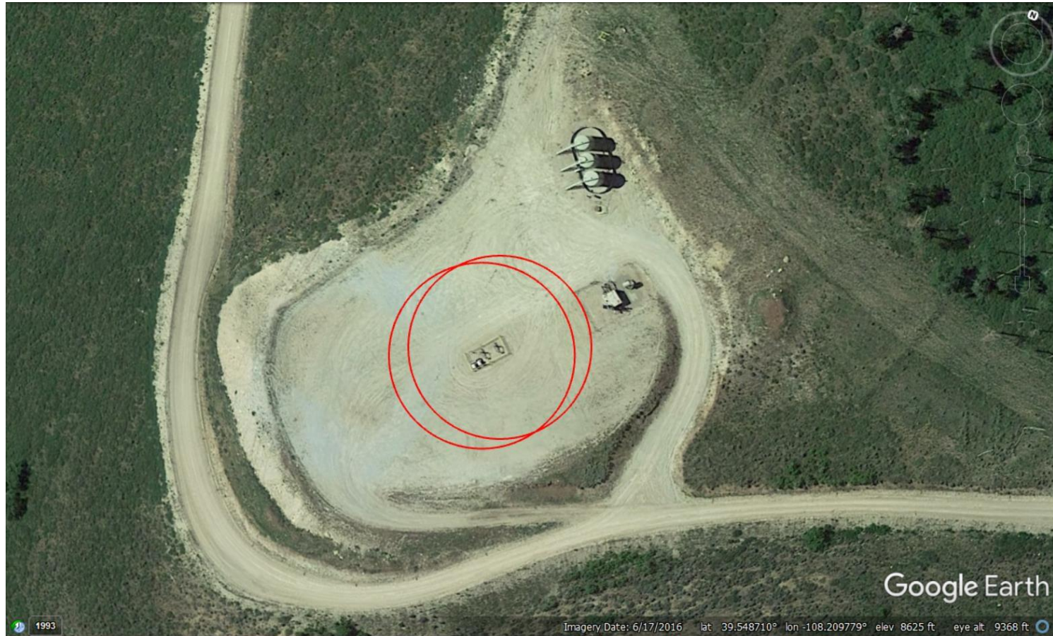
Photo 2: Photo taken from doc. #696202107. Google Earth aerial imagery. Photo shows areas of the Location not needed for production operations have not been reclaimed. Red circles represent a 75 foot buffer around producing wells.
