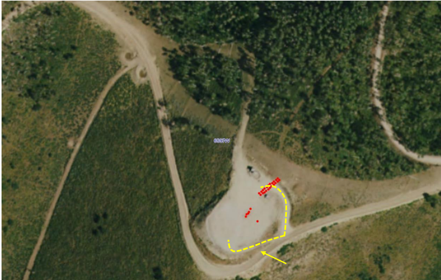
Photo 1: Photo taken from doc. #696202107. 2019 COGIS Aerial imagery. Photo shows two access points/roads have been constructed on the south end of the Location (dotted yellow lines). Previous inspection required reclamation of areas not needed for production on the south end of the Location, and the western traveling access road (arrow) also on the south end of the Location; It was observed that reclamation has not been conducted.
