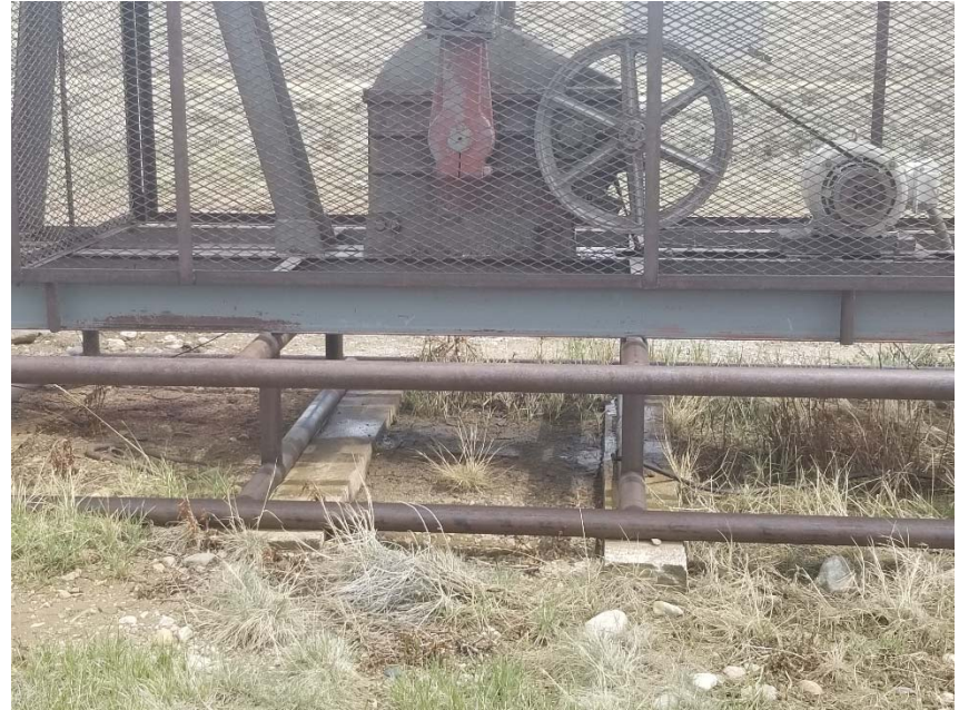
Photo 2. Stained soil under pump jack.
