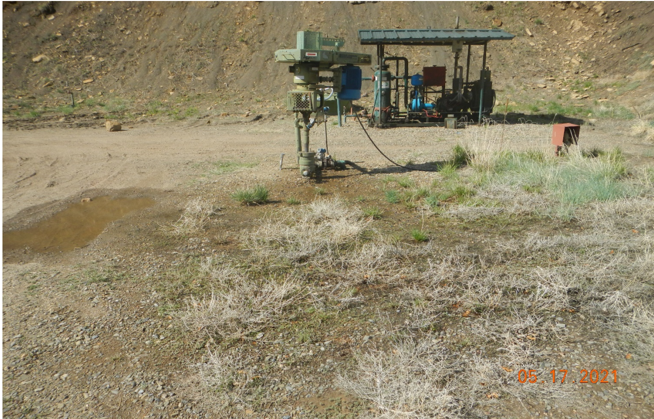
Photo 3. There is a water leak at the wellhead that needs to be repaired.
