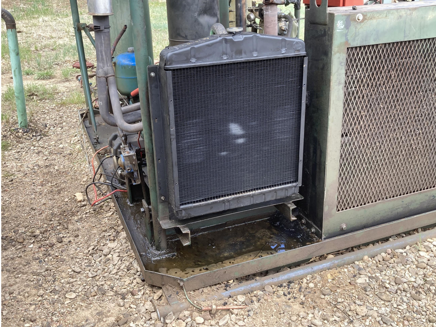
PHOTO 1: THE FLUID ACCUMULATION THAT WAS FOUND INSIDE OF THE CONTAINMENT SKID OF THE LIQUID RING COMPRESSOR WAS REMOVED.
