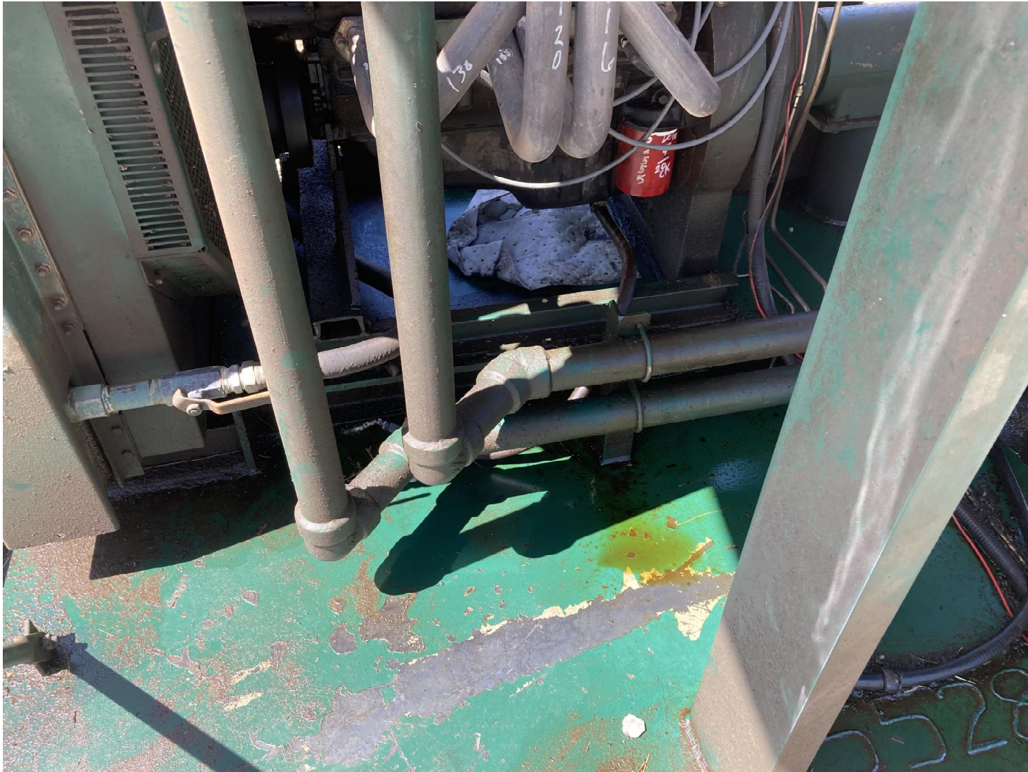
PHOTO 1: THE LEAKS ON THE COMPRESSOR WERE REPAIRED. ALL FITTINGS ARE SECURLY FASTENED. THE FLUID ACCUMULATION WAS REMOVED FROM THE CONTAINMENT
