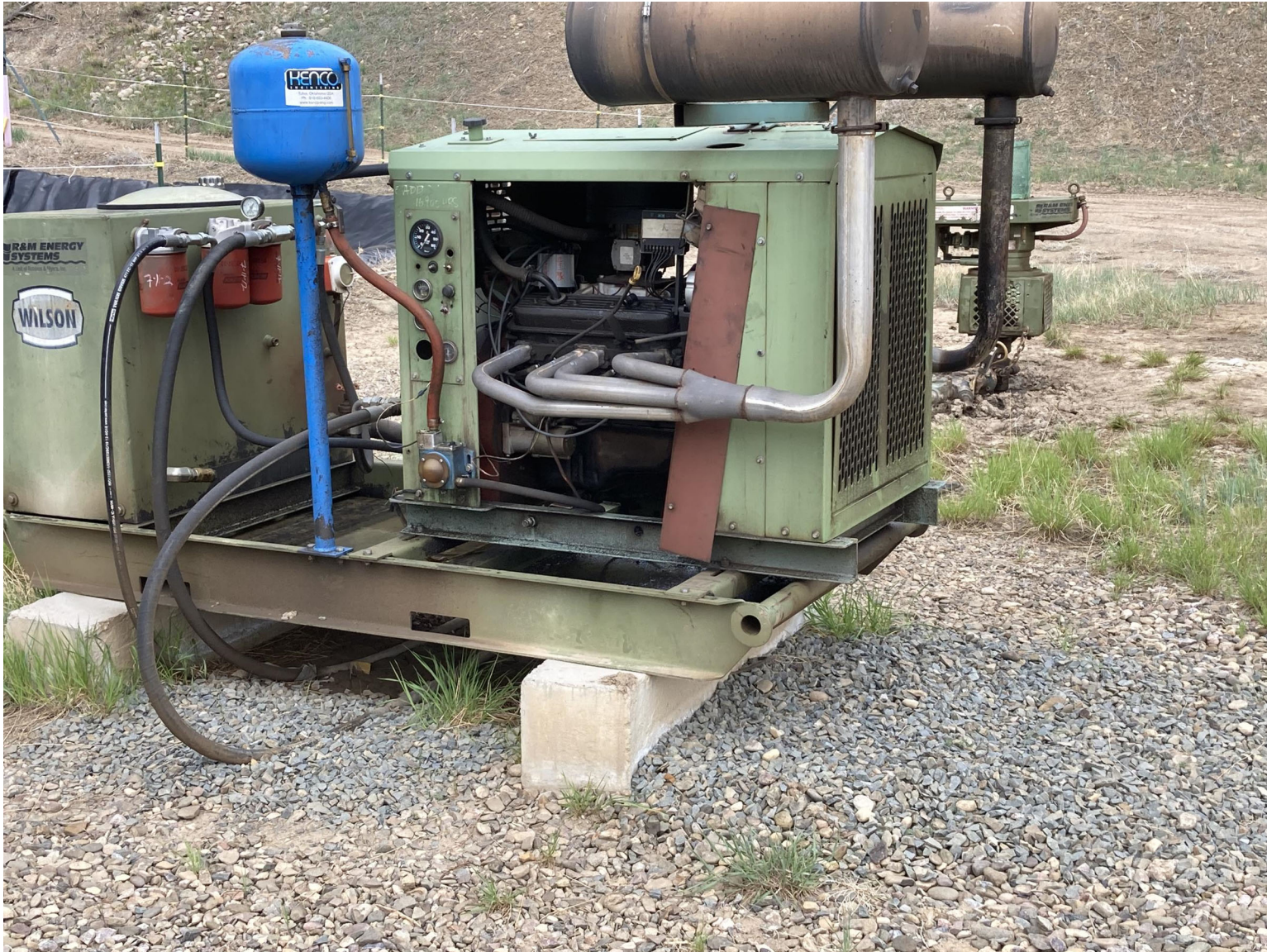
PHOTO 2: THE LEAKING MUFFLER ON THE ENGINE SKID WAS REPAIRED AND THE IMPACTED SOIL ON THE GROUND WAS REMOVED.
