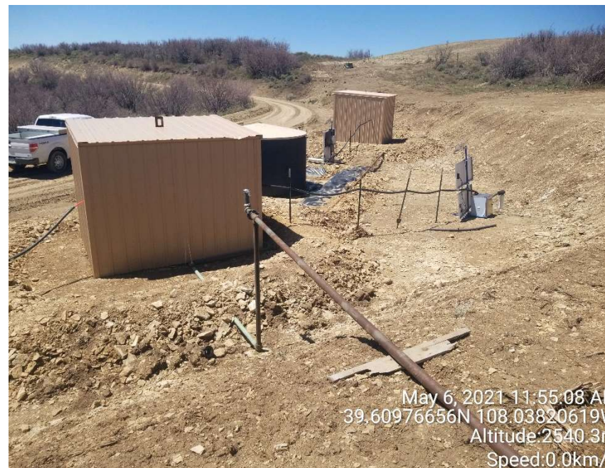
Overview of the two structures and steel AST. Note the 2-inch steel pipeline that is attached to both of the structures on location.
