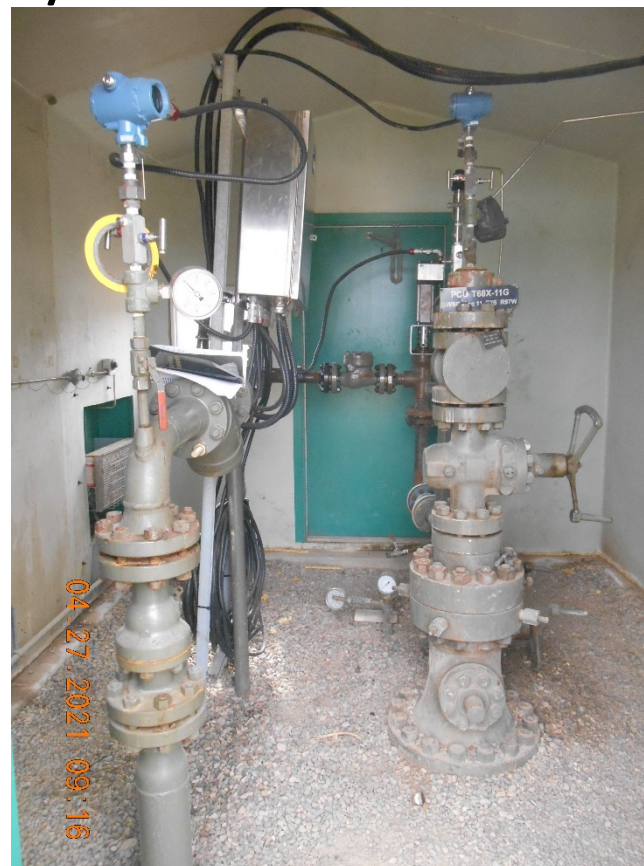
Injection wellhead. Shut in.
