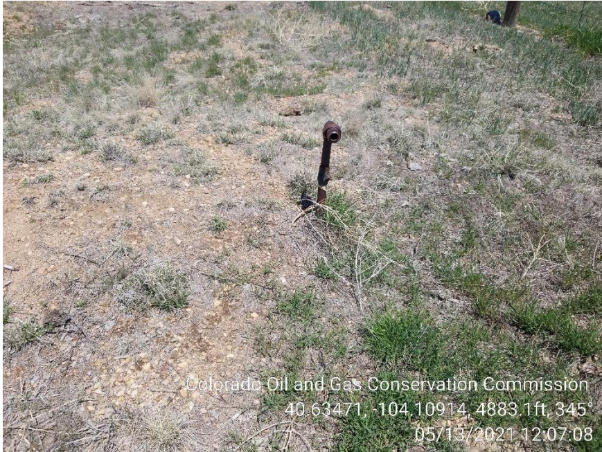
Photo 3 – Unmarked Riser South of Wellhead
