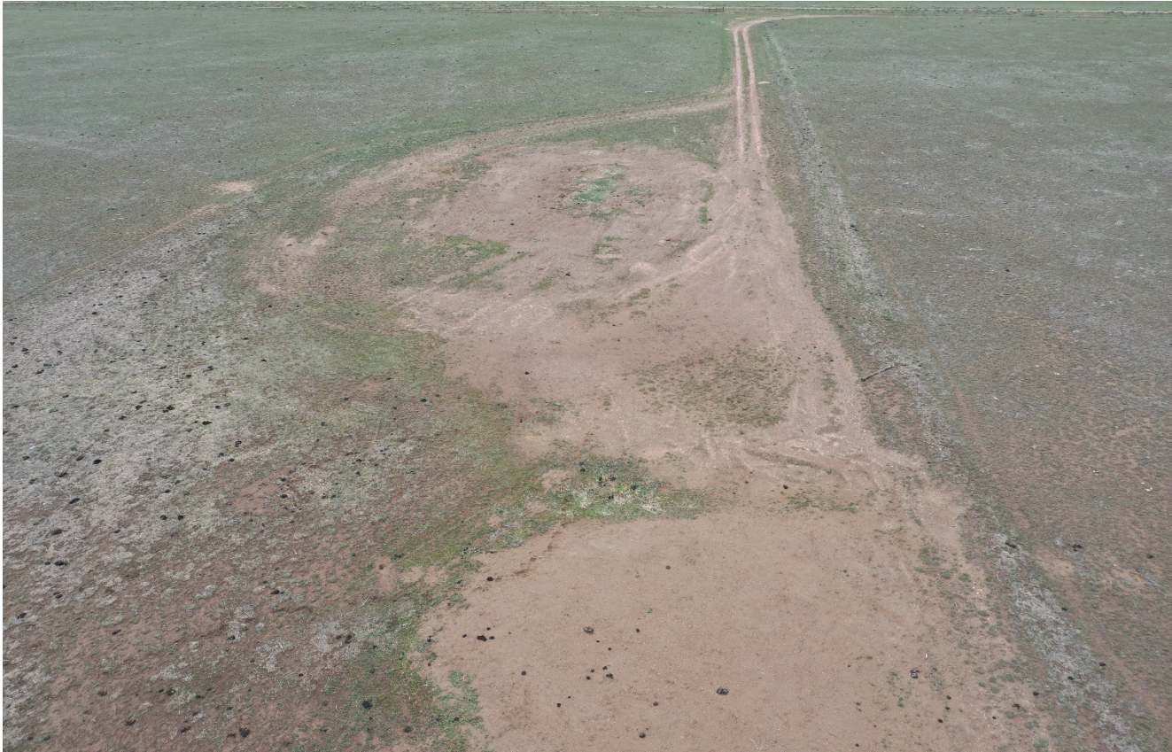
Photo 9. Facing down toward the location. The location remains mostly devoid of vegetation growth. There is no indication that reclamation was performed.
