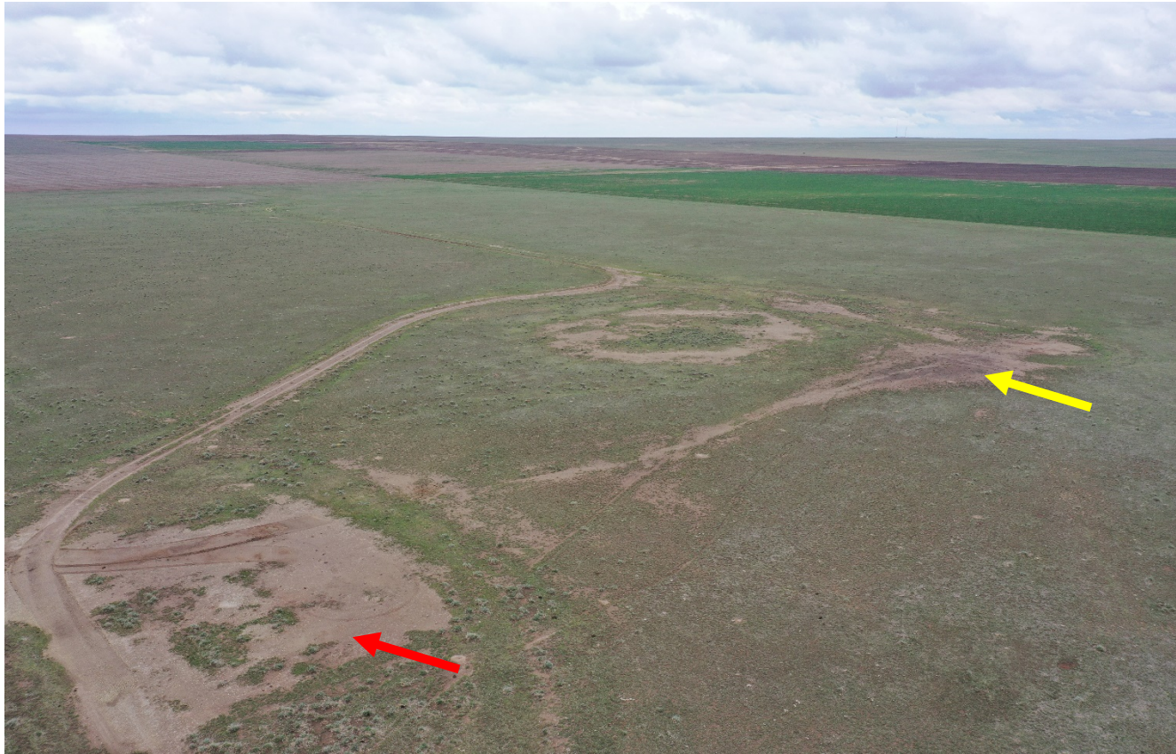
Photo 1. Drone aerial photo facing southwest toward the location. Red arrow points to tank battery site. Yellow arrow points to the well site. The vegetation has not re-established in the disturbance area. Reclamation has not been completed.
