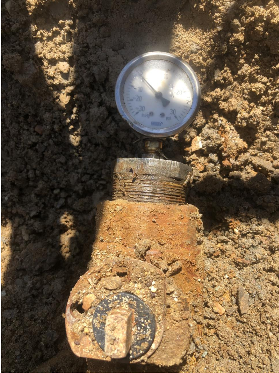
Plumbed bradenhead to surface for monthly monitoring to comply with Rule 341.
