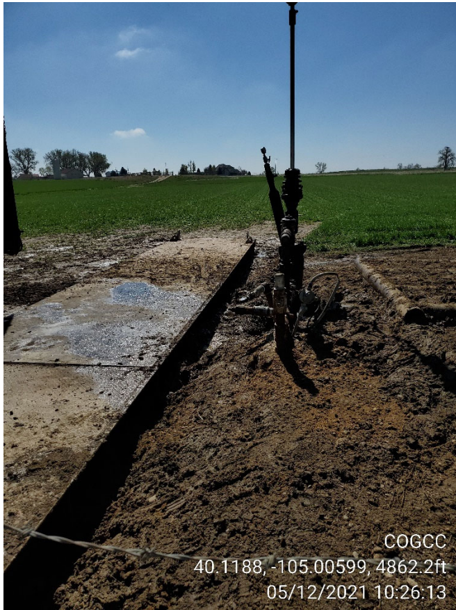
Photo 3 Well with workover platform
