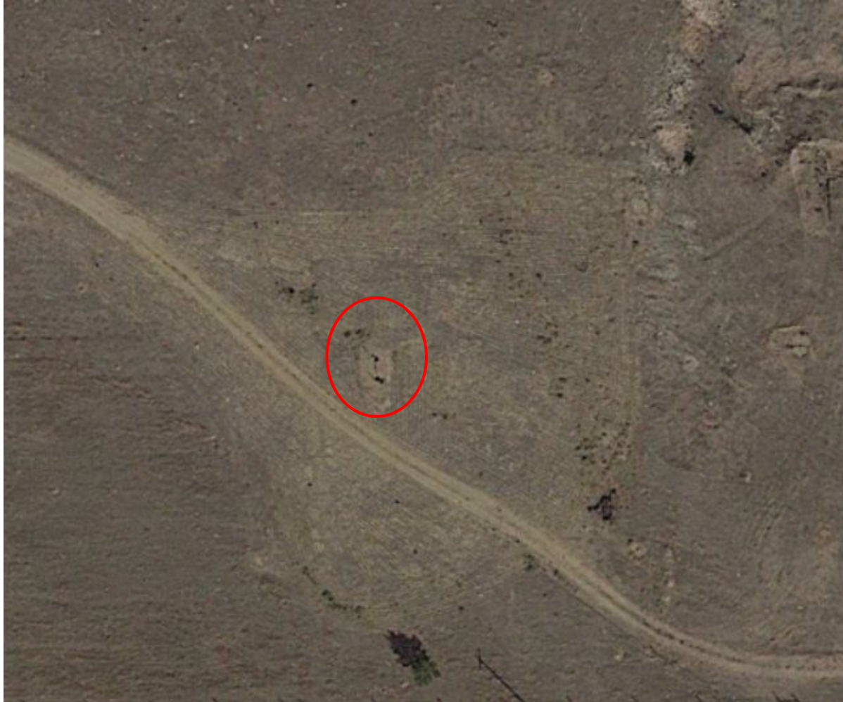
Photo 2. Google Earth aerial from 9/29/2020 illustrating conditions after plugging and abandonment. Photo illustrates the Operator has failed to remove all equipment.
