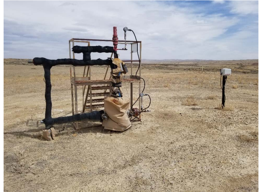
Photo 2. No bradenhead access apparent.
