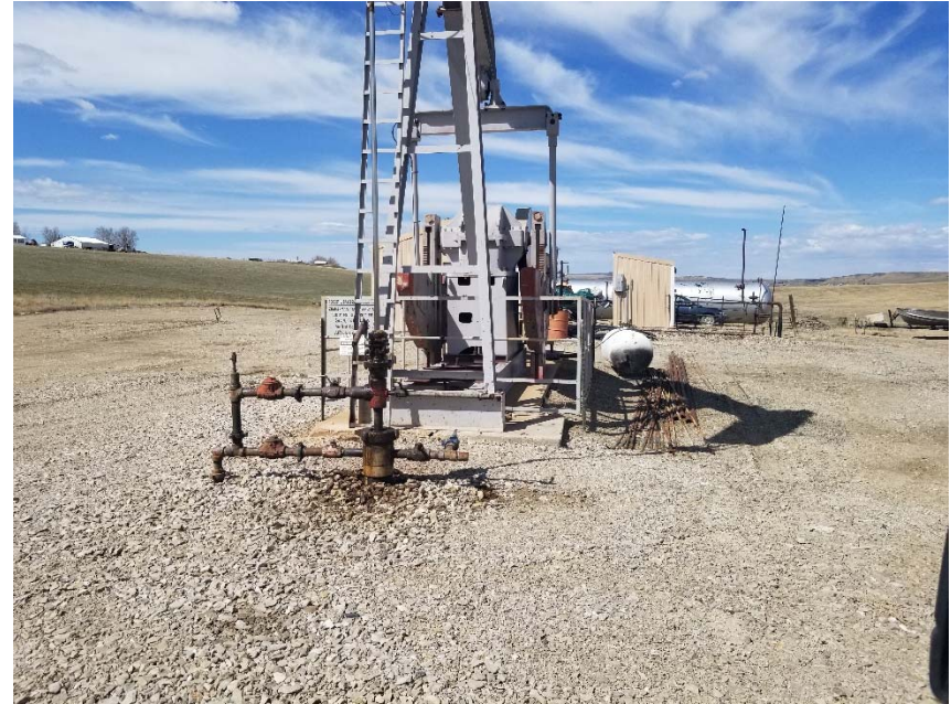
Photo 2. No bradenhead access apparent. Stained soil at wellhead. Tubing stored at wellhead.
