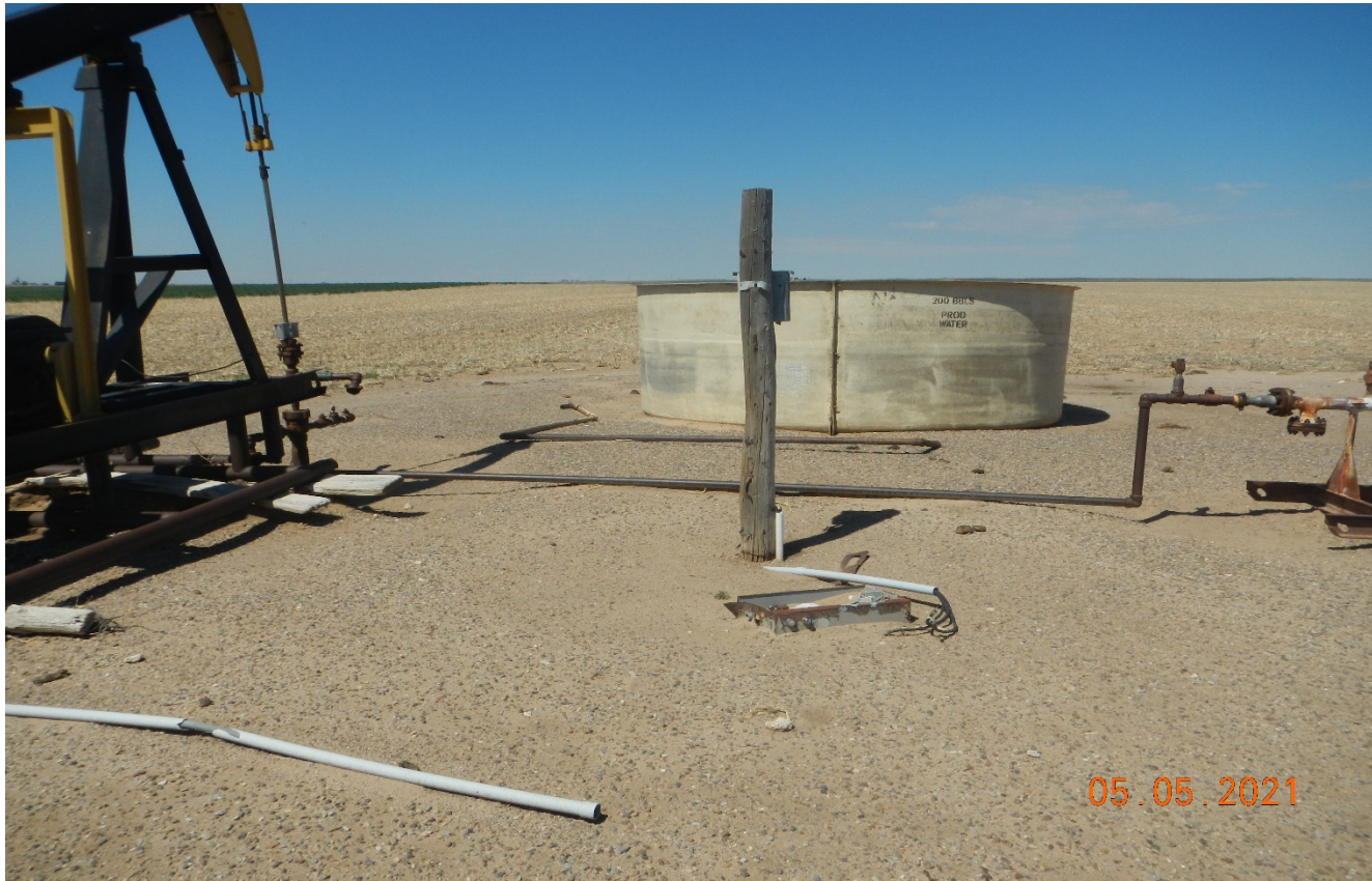
Photo 6. There is exposed electrical wire on the ground and panel box. All unused supplies and equipment need to be removed.
