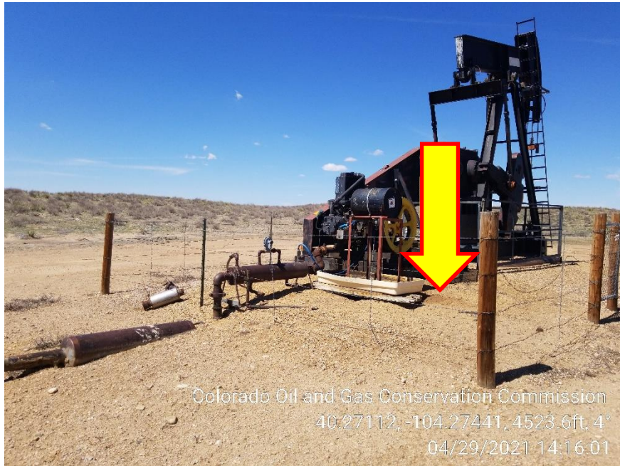
Photo 1 – Pumping Unit – Stained Soil
