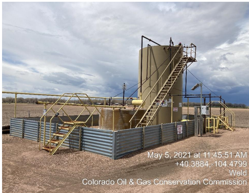
Photo #1 Tank Battery
