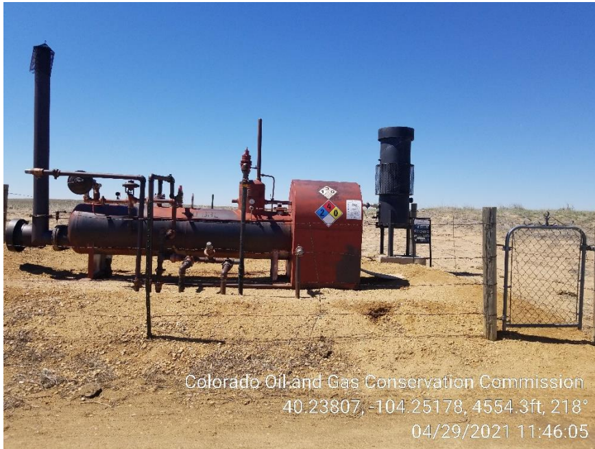
Photo 5 – Separator and ECD
