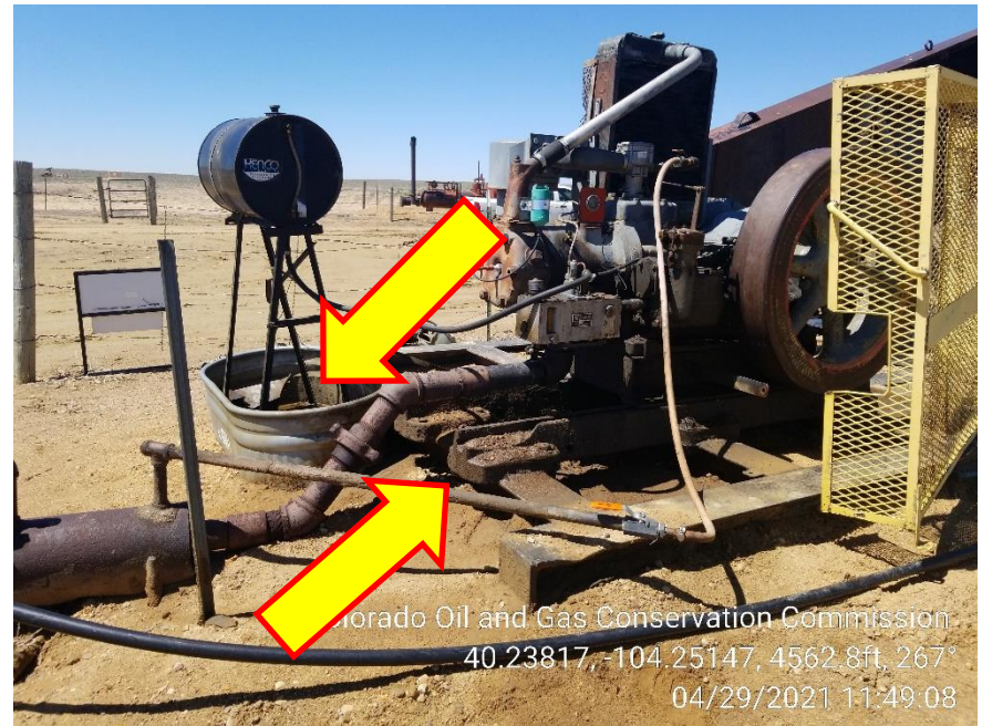
Photo 10 – Stained Soil at Gas Engine and Wildlife Netting missing
