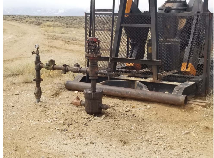
Photo 2. No bradenhead access apparent.
