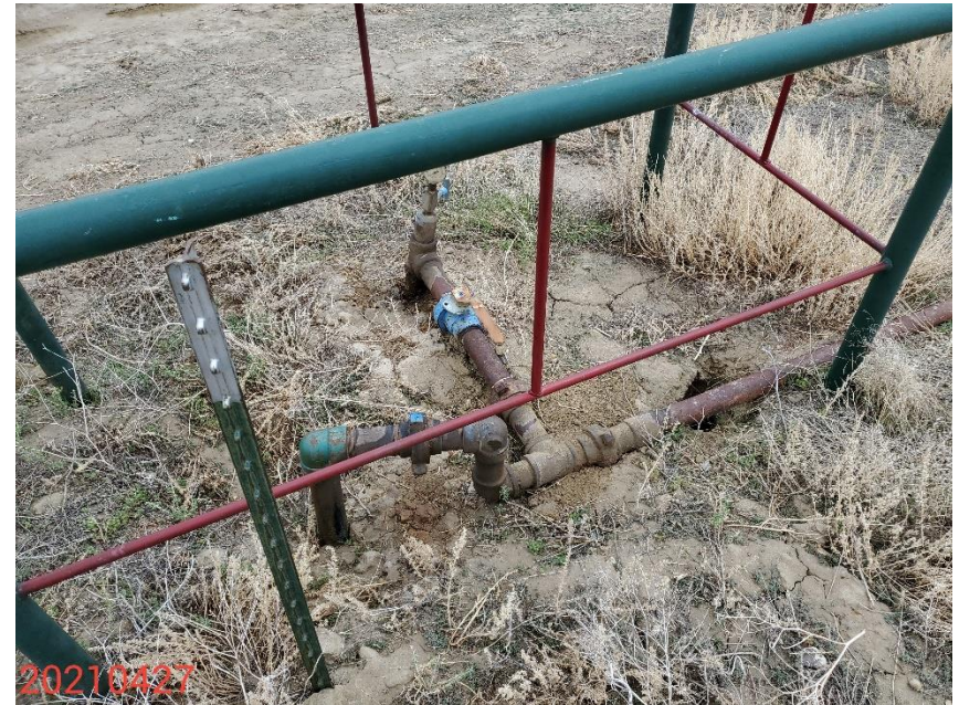
Photo 4: Photo taken from the flowline riser on the north end of the Location. Integrity issues (corrosion/leaking) were observed on the flowline/flowline system.
