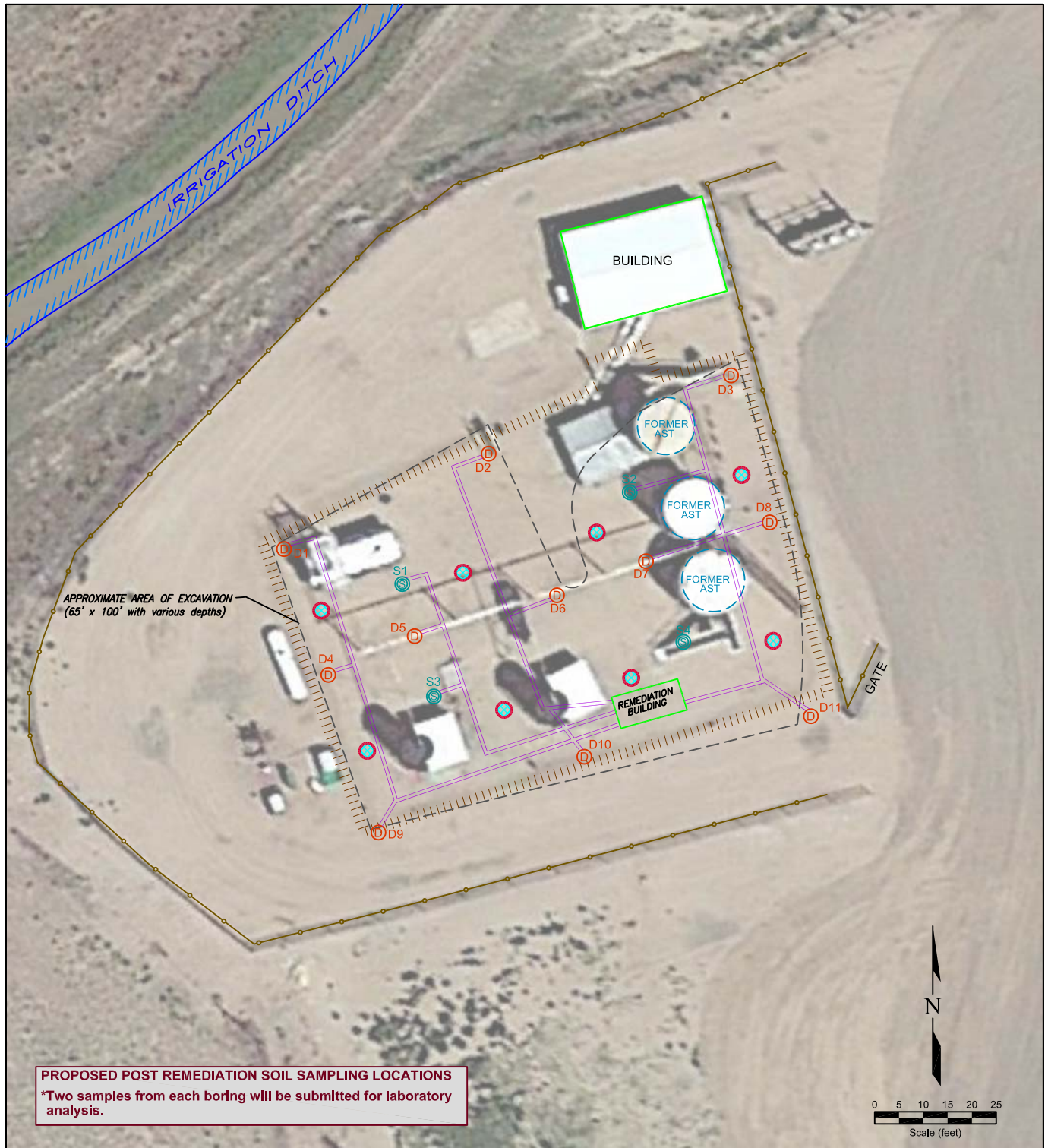
Figure 2 AS-BUILT AS/SVE LAYOUT WITH PROPOSED POST REMEDIATION SOIL SAMPLING GREAT WESTERN OPERATING COMPANY, LLC PIERCE CENTRAL STATION SESE Sec 22, T8N, R66W ~ 40.6438°, -104.7572° Weld County, Colorado
