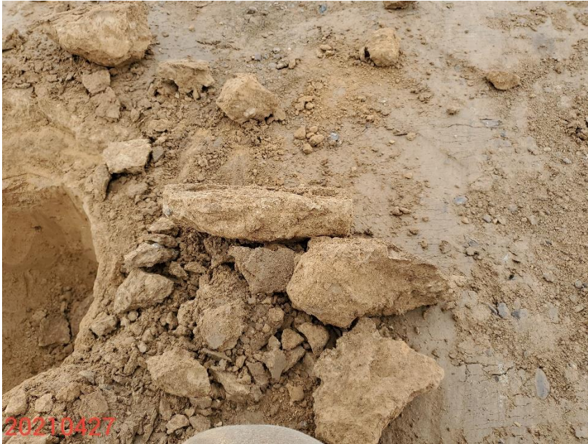
Photo 9: Reclamation Specialist dug a test pit on the Location to determine compliance with compaction alleviation requirements; comaction issues were observed in the top 4-5 inches of the soil; it is unclear if compaction alleviation has been performed per COGCC Rules.
