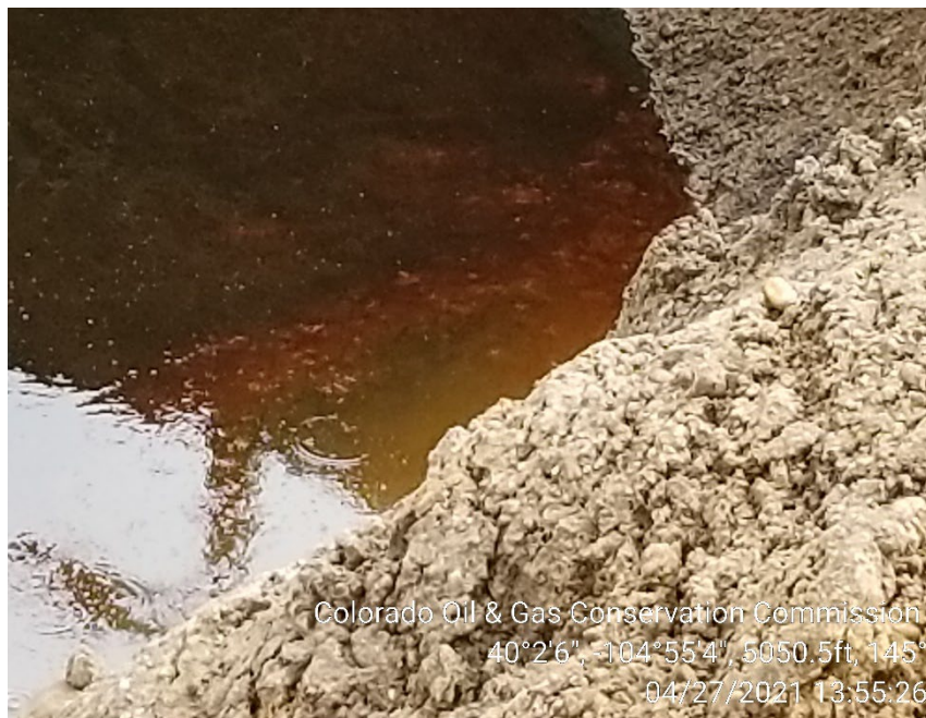
Close up of oil floating on groundwater in the excavation
