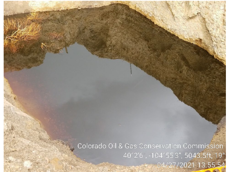
Oil floating on groundwater in the excavation
