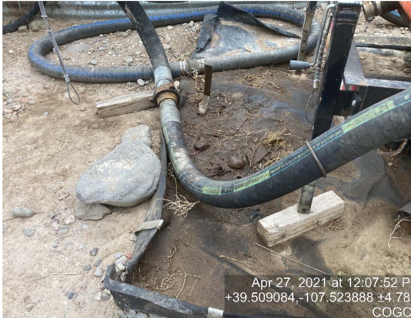
Staining and secondary containment failing
