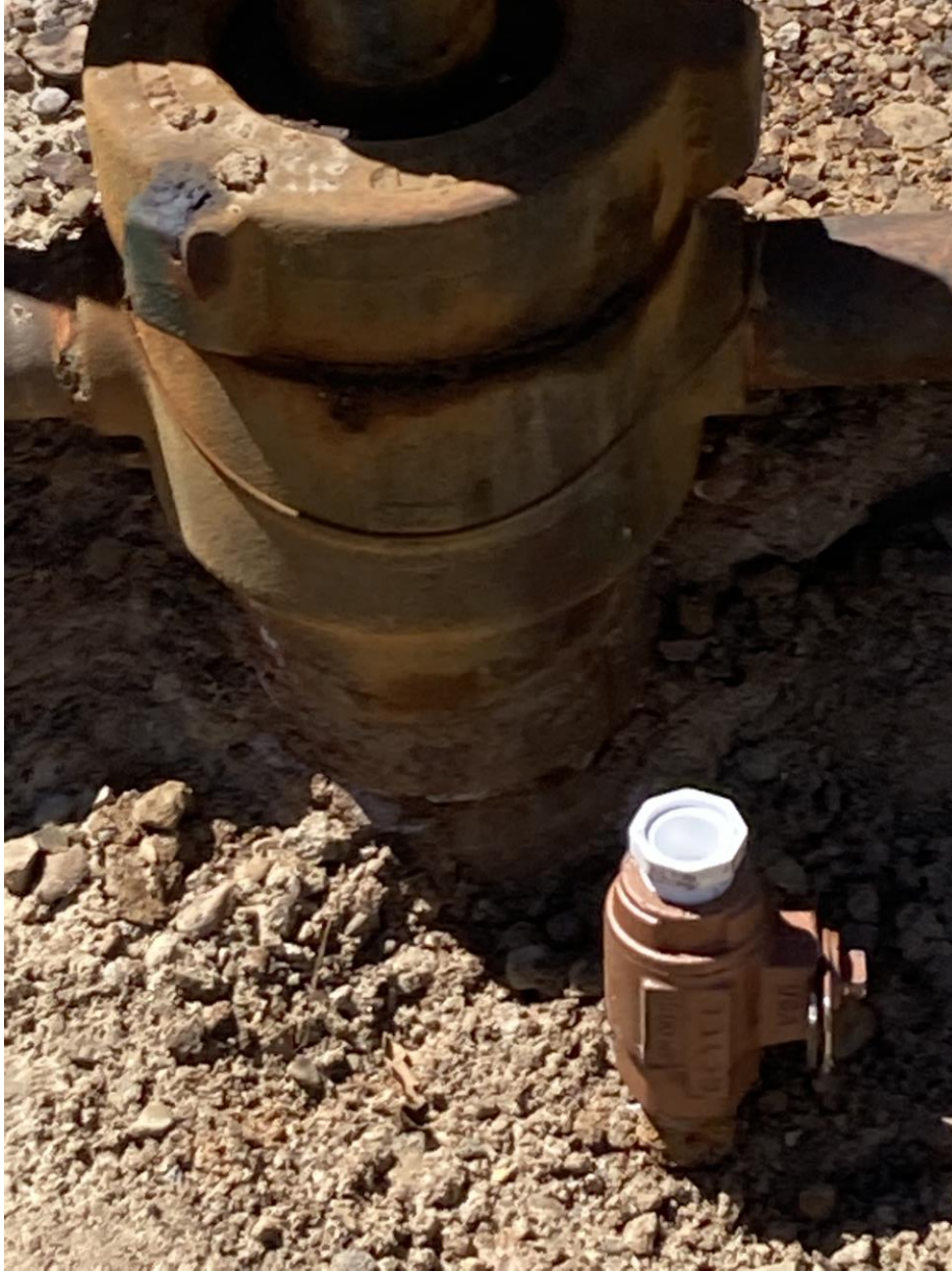
Plumbed Bradenhead to the surface for new Rule 341.
