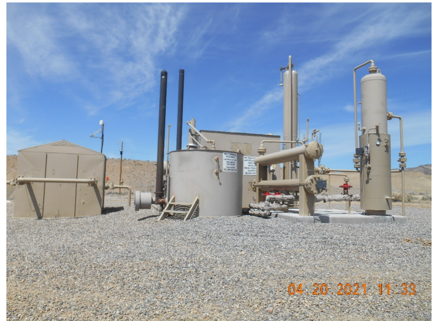
Separator, Dehydrator, Meter housing and Tank
