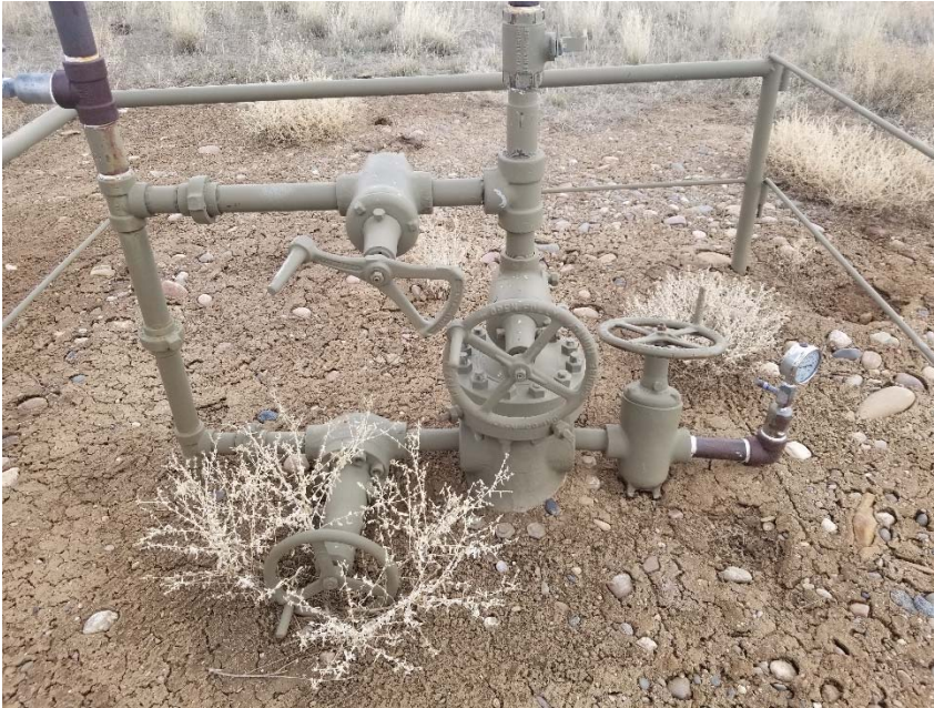
Photo 4. No bradenhead access apparent.
