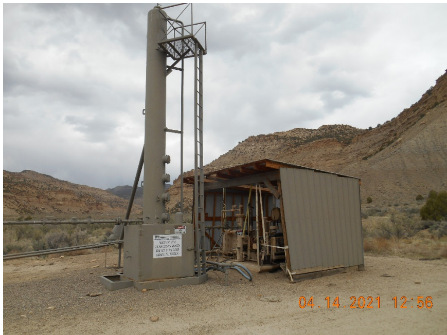
Dehydrator and Compressor housing.
