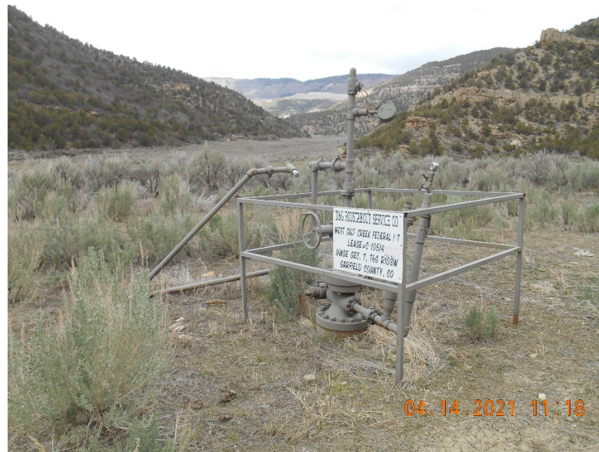
Wellhead with fence and sign
