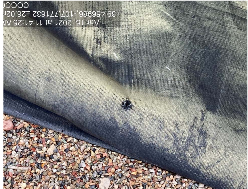
Multiple holes in containment
