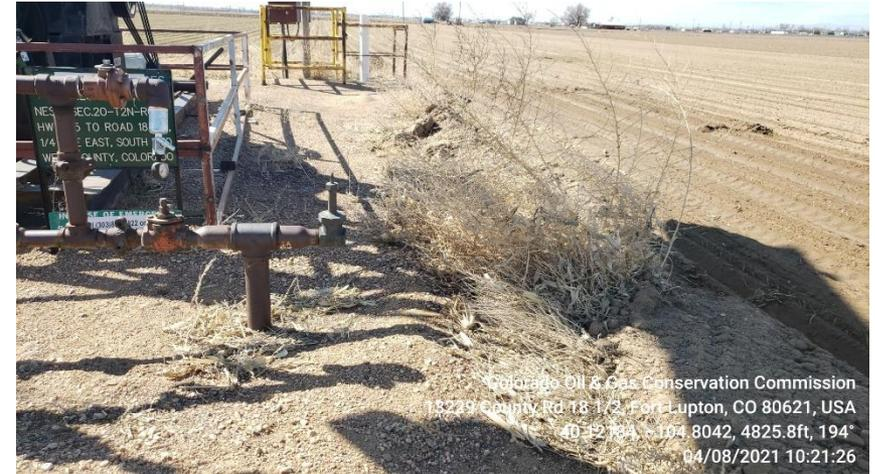
Photo 5 braden head gauge missing cover and needle is missing.
