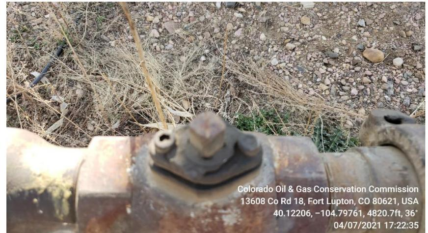
**Photo 3 Valves on WH are closed, broken gauge.**
