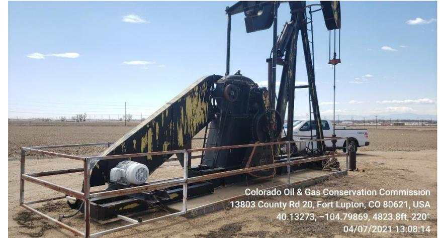
**Photo 5 braden head gauge not in working order missing cover.**
