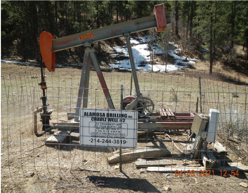
Chavez #2 pump jack and well head.
