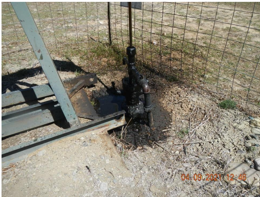
Oil puddle around well head and stained/wet vegetation and soil.
