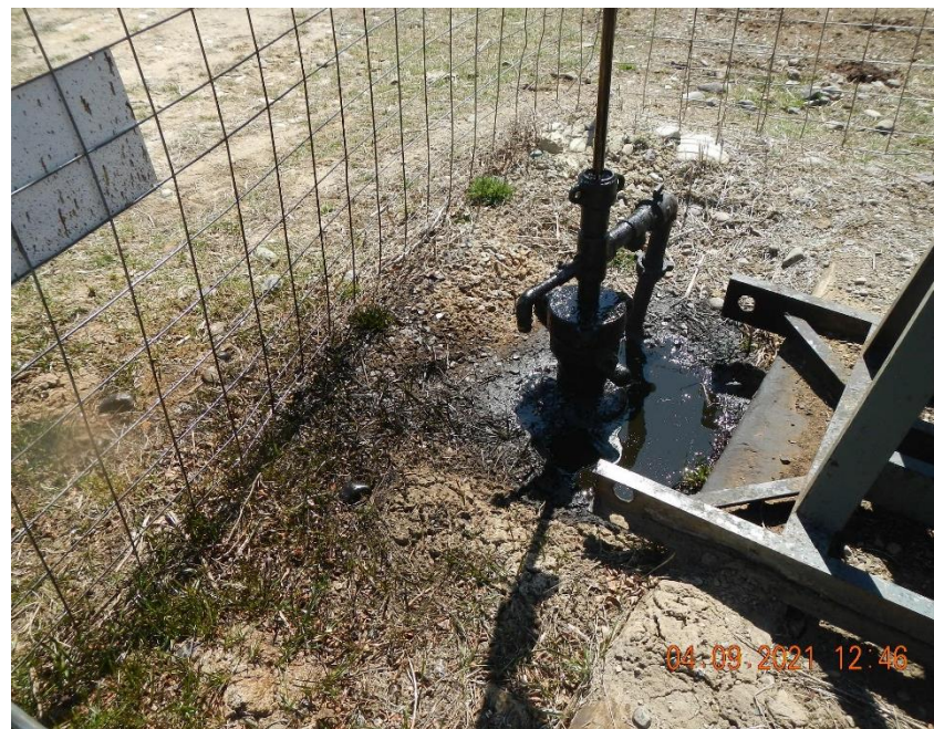
Chavez #1 well head is wet and stained. Surrounding area is wet and stained with oil.
