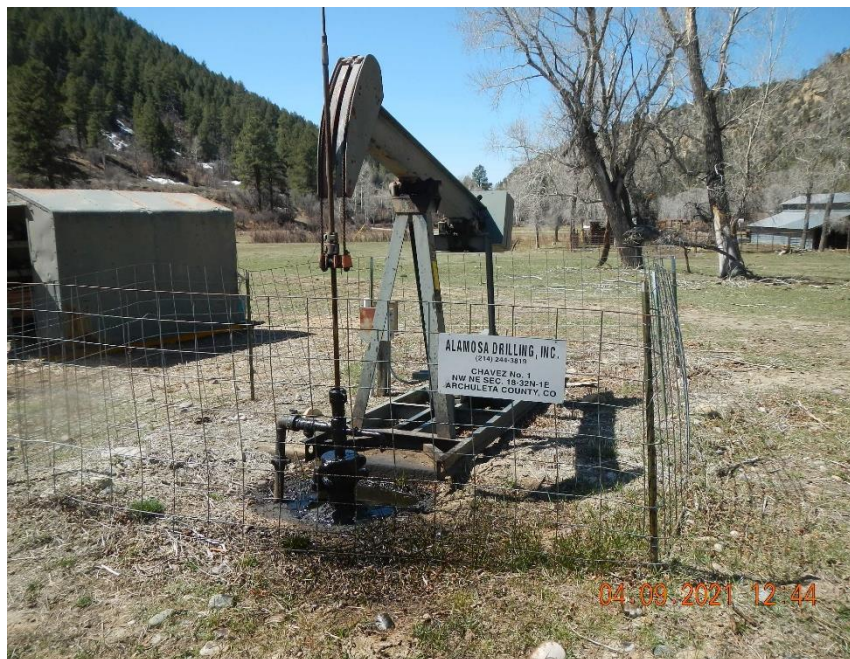
Chavez #1 well head and pump jack with oil impacted soil and vegetation.
