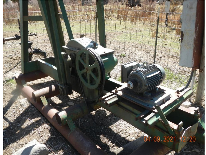
Drive belts on pump jack have broken. EPS staff shut down power to electric motor.
