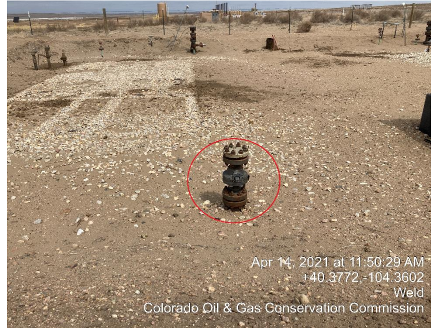
Photo #2 Riser is unmarked & not locked out
