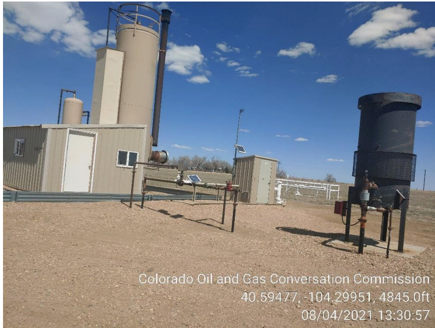
Photo 3 – Heater Treater and ECD
