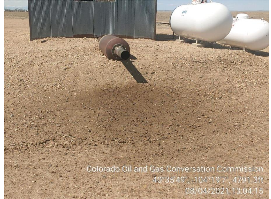
Photo 6 – Exhaust – Stained Soil
