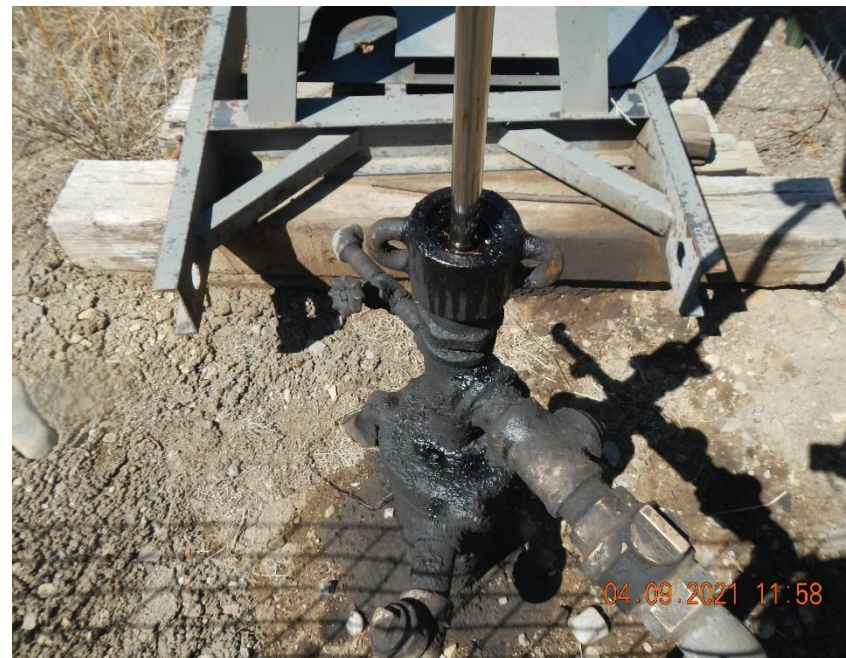
Well head is wet and surrounding soil is stained.
