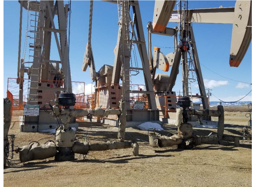
Photo 6. Incomplete wellhead signs.
