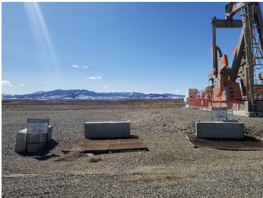
Photo 3. Wellhead signs without all necessary information.
