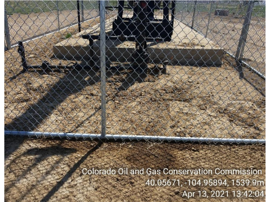
Photo 4 Stained soil around well head.
