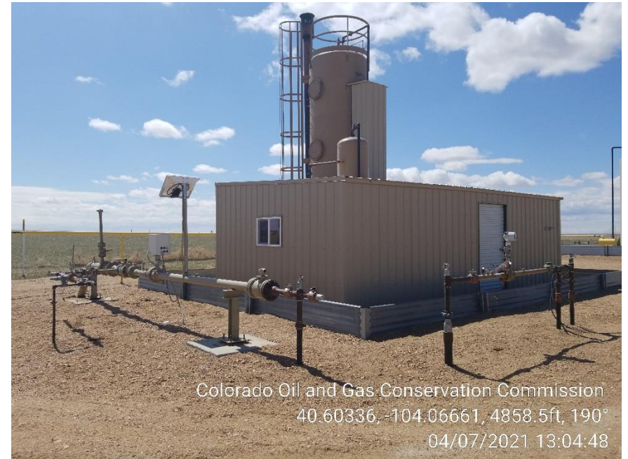
Photo 4 – Heater Treater
