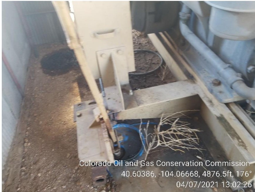
Photo 11 – Stained Soil at Gas Engine
