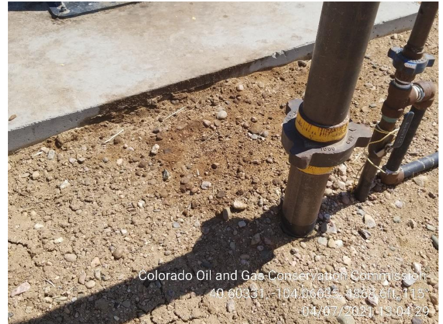
Photo 16 – Stained Soil at Flare
