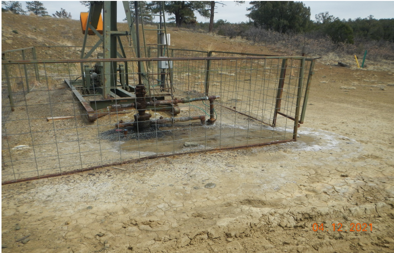
Photo 3. There is produced water leaking from the wellhead.
