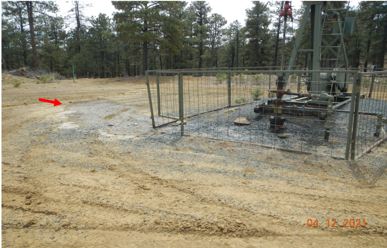
Photo 5. There is produced water leaking from the wellhead.
