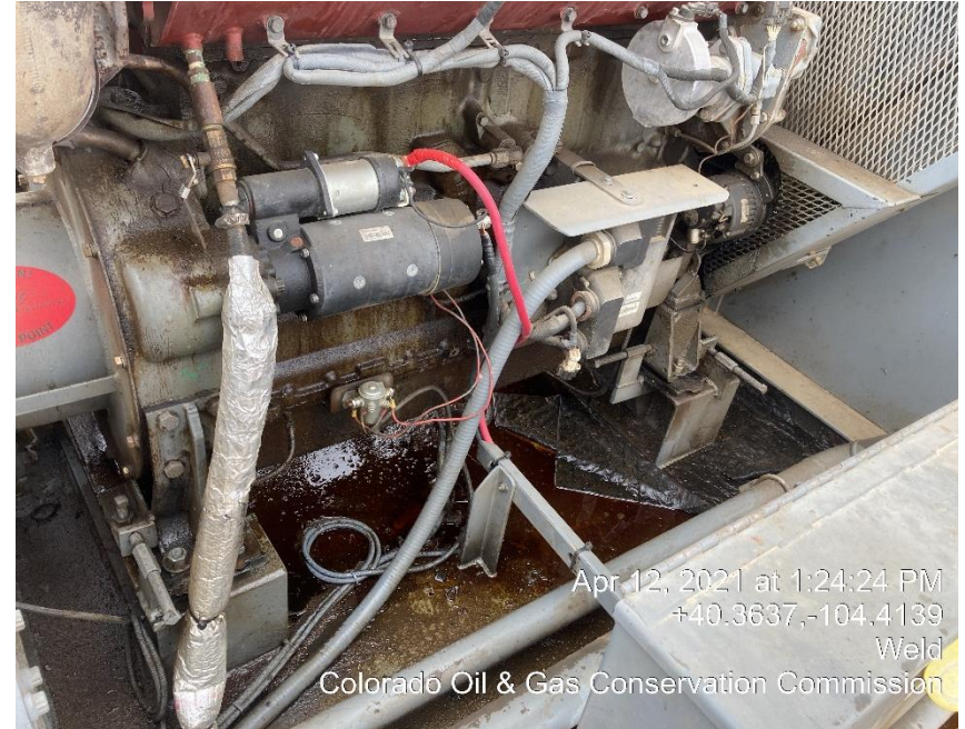
Photo #3 Mechanical Conditions & Oily Skid
